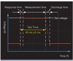
Applied Voltage Waveform at Fastest Test Time
